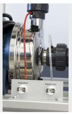
The equipment has pressure ports prepared to be able to perform the analysis and calculation of the characteristic curve of the pump.
