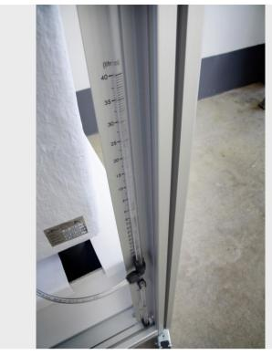
The upper tanks have calibrated rules to facilitate the work of the student in the flow measurements.
