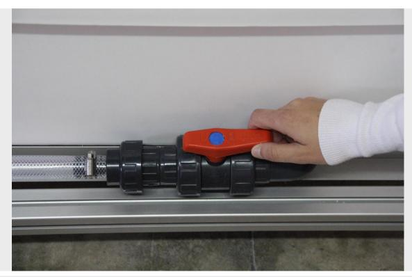
The lower tank has a coupling for easy filling and emptying of the equipment.
